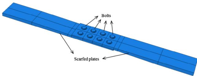
**Fig. 2.** The scarf bolted joint.
