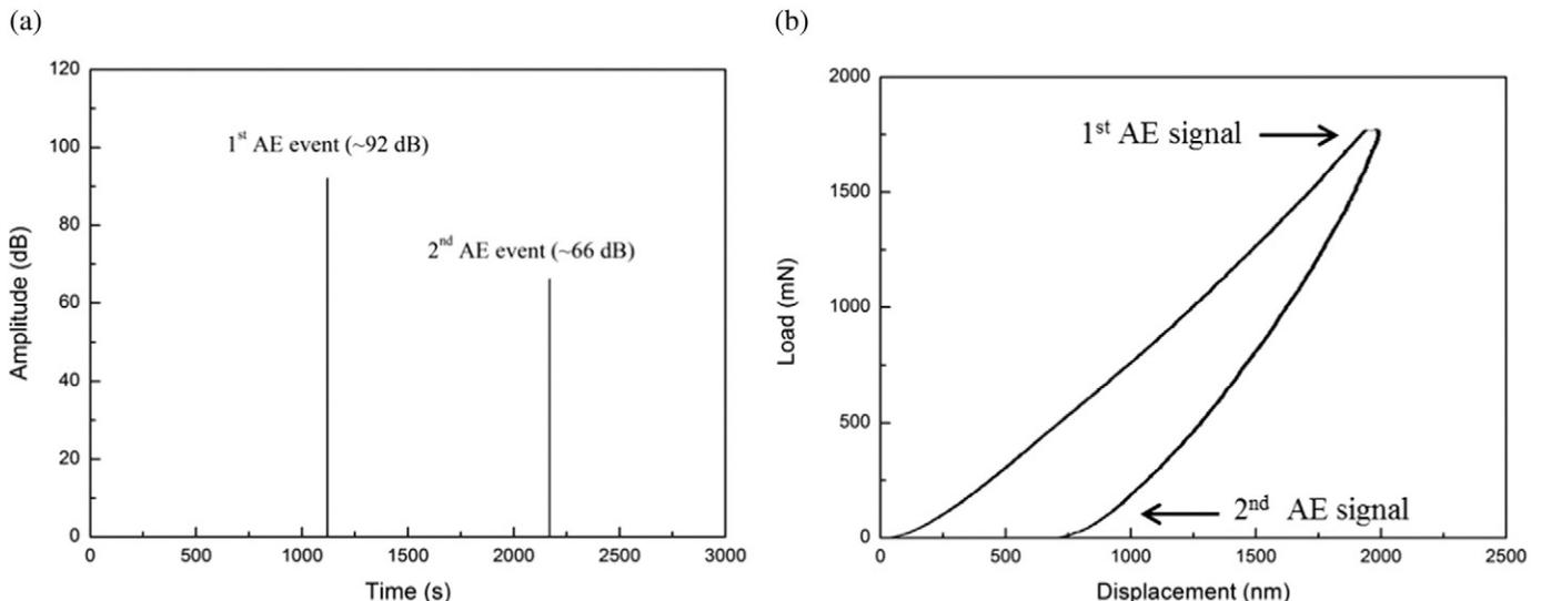
Fig. 9. (a) Time history graph and (b) the  $P$ - $d$  curve of a particular indent on the Cu/Ti/SiO<sub>2</sub>/Si sample.
