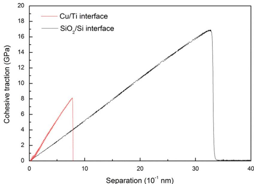
**Fig. 4.** Cohesive traction-separation relations of the Ti/Cu and SiO<sub>2</sub>/Si systems under tensile loading at 300 K.
