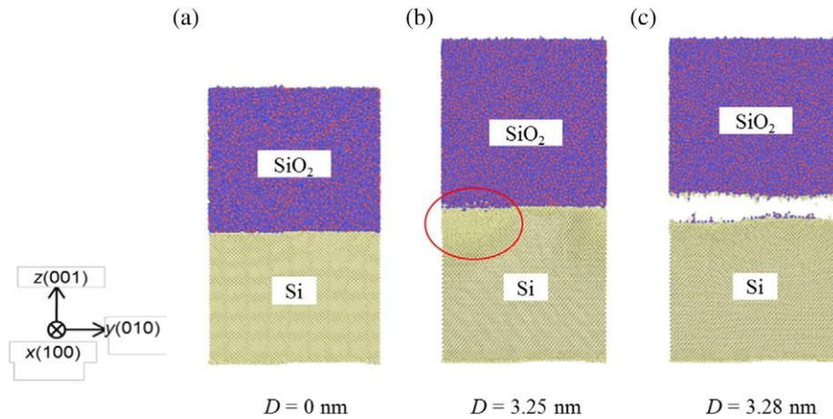
Fig. 6. The atomic configurations of the SiO<sub>2</sub>/Si systems under tensile loading at *D* of (a) 0, (b) 3.25 and (c) 3.28 nm.
