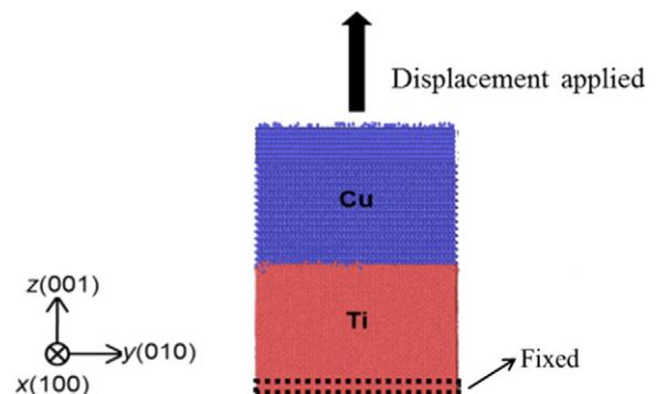
Fig. 1. Computational cells of the Cu/Ti system.
