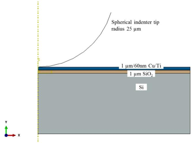
Fig. 2. Initial configuration of the FEM model of the Cu/Ti/SiO<sub>2</sub>/Si system
