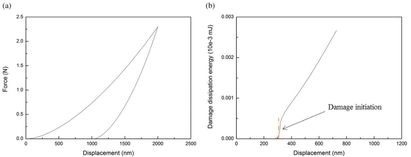
Fig. 8. (a) The  $P$ - $d$  curve of the Cu/Ti/SiO<sub>2</sub>/Si system and (b) the corresponding damage dissipation energy graph obtained from the FEM simulation.
